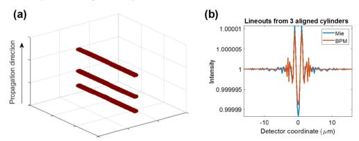
Fig. 4. Simulation of three axially aligned cylinders. (a) Illustration of cylinder geometry and propagation direction. (b) Lineout of the scattered intensity. Here, the pixel size was 0.25 $\mu$ m, the cylinder diameters were 2  $\mu$ m, and the photon energy was 0.3 keV. The cylinders were displaced –8  $\mu$ m, 0  $\mu$ m, and 12  $\mu$ m from the center, respectively. Here, the mean difference was <10<sup>-5</sup>.
